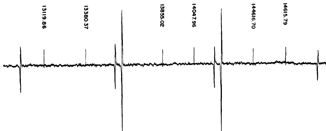
Figure 4. ESR spectrum of the trifluoromethyl radical from P(CF_3)_3 in a cyclopropane solution at -80^\circ . The central lines of the quartet are split by second-order effects.
